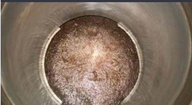
Reconditioned Barrel of the Hydraulic Jack
