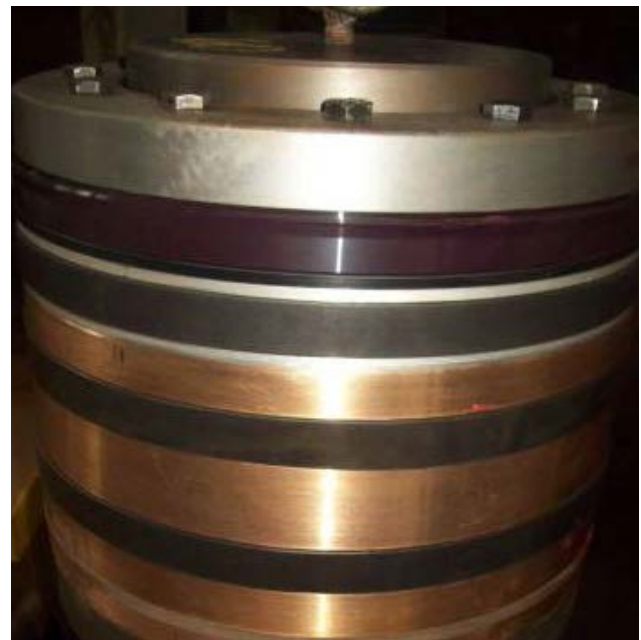
Chesterton® AWC 800 22K Piston Seal and 18K GNF/MWR Coil TB Bearing Bands on the Jack Ram
