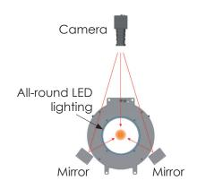
Thanks to a mirror system and a very powerful all-round lighting that eliminates shadows, **every vegetable is subjected to a perfect 360° analysis.** The optical system generates 3 immaculate high-resolution images of each carrot. These can be displayed immediately on the computer screen to check the error detection.
