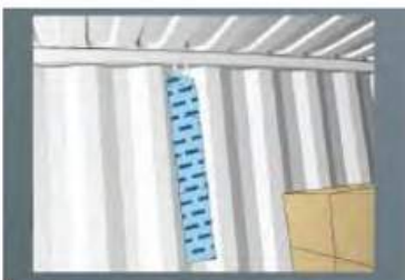
4. Hang desiccant from ceiling hooks
