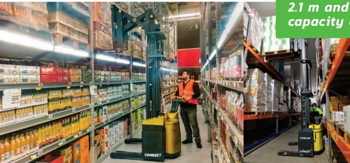
The first purpose built pedestrian reach stacker with to operate in a VNA aisle of just 2.1 m and with a lift capacity of 2000 kg.
