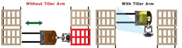
The tiller can be turned to the left or right, allowing the operator to remain at the side, while maintaining full steering control. Standing to the side of the stacker eliminates the risk of being trapped or crushed, while allowing the COMBi-WR4 to operate in very narrow aisles.
