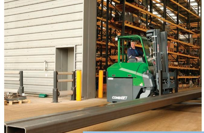
Counterbalance operation combined with the ability to carry long loads, such as timber or steel beams, in sideways mode makes the COMBi-CB the most versatile all-round forklift available.
