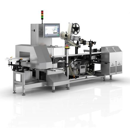
When processing food in particular, you are well advised to weigh, label and inspect the product for metallic foreign bodies in the same process step. This configuration covers all those functions and unites them under a central control. It is mostly applied to label thermoformed trays or flat cartons on the top and bottom.
