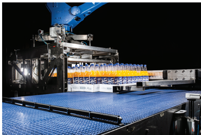
The automatic pusher for multipack is fully integrated in the MOTOMAN robot's control system.
