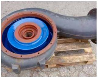
The MetaLine process is suitable for the protection of complete metal components as well as the repair of existing rubber linings and parts.
