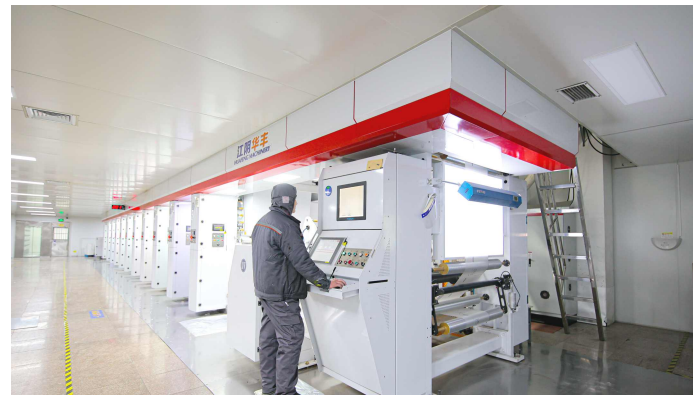
10-color gravure printing machines for reverse print, surface print and lacquer coating. Computer-controlled registration. Online inspection system.
