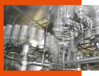
The magnetic filling valves ensure safe production and beverage integrity.
