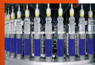
Rollsleeve has a continuous throughput and automatically controls the flow of containers entering and exiting the machine.
