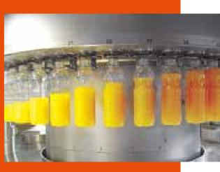
Each capping head is individually adjusted and constant torque is ensured.
