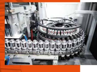
Direct transfer from oven to mould via transfer wheel reduces overall production time, and is supported by reliable open/close gripping control.
