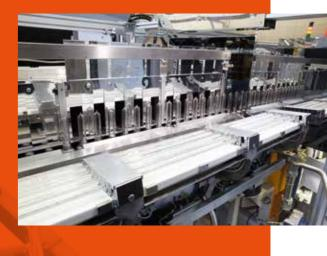
The in-oven neckorientation mechanism keeps the preferential heating profile aligned with bottle specs.
