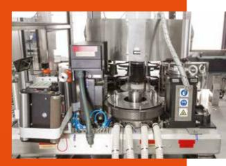
The carousel transmission enables the application of wraparound labels for both round and irregularly shaped containers.
