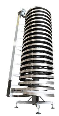
The AVo, which is reversible, provides vertical accumulation and starts buffering. Products enter the AccuVeyor AVo on a LIFO basis, and once the downstream process is running again, the AVo reverses, and via a second switch, the products are brought back into the production line again. This "off-line" buffering system compensates for downstream stops and significantly improves the overall production efficiency.
