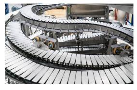
The next generation of dynamic accumulators, designed by AmbaFlex, solved this issue. We designed an AccuVeyor that doesn't transfer the product itself but the belt it sits on. With a system called the Belt Transfer Unit, the machine lifts the track instead of the product. This ensures that every product stays on the exact same spot of the belt, keeping it in perfect condition.
