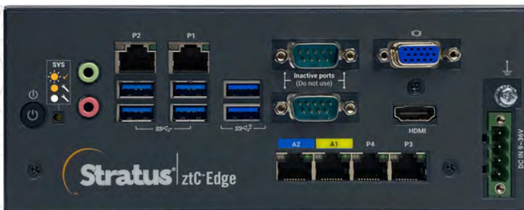
Figure 3. Some modern Edge Computing platforms are industrial grade, such as the ruggedized, Class I Division 2 (CID2) certified Stratus ztC Edge Computing platform, which can be installed in hazardous locations, with the PLCs, in the same control panel without special accommodations for temperature, humidity or vibration protection.
