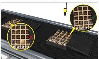
Al tools ensure all pieces in an assortment are present and undamaged.
