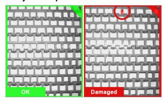
Continuous visual belt inspection uses Al-enabled technology to reduce the risk of food contamination due to undetected broken belt links.
