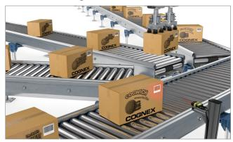
DataMan barcode readers quickly read barcodes at various heights and angles to facilitate automatic sorting.
