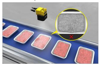
Al-based vision systems check the integrity of film seals on trays and read product labels and codes to prevent mislabeling.
