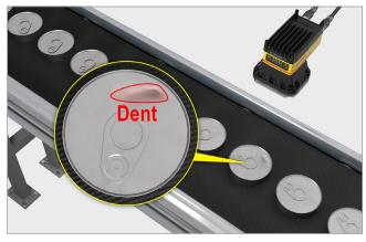
Al-based vision systems and software identify defects on challenging food and beverage packaging surfaces.
