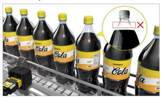
In-Sight 2D vision systems measure liquid volume for proper filling.
