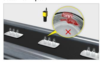
Al-enabled technology detects variable defects in threaded necks of glass containers.
