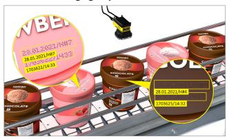
Al-based OCR solutions quickly read alphanumeric codes on multi-part packaging to ensure components match.
