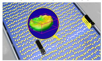
3D displacement technology ensures product meets size and dimension requirements to ensure even cooking.
