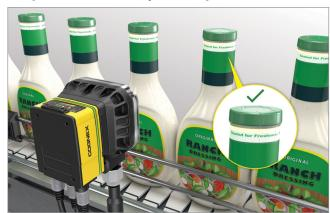
Machine vision technology detects safety seal defects and limit product recalls.
