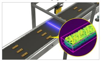
3D vision systems inspect food elements for damage and confirm dimensions and volume.
