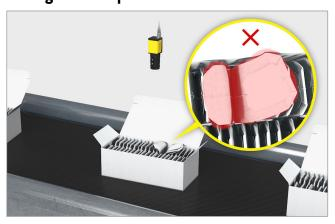
Al-powered technology ensures that tea bags and cartons are correctly packed.
