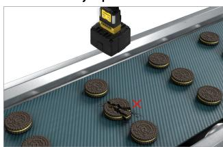
Machine vision systems detect damage and ensure consistency in size, shape, color, and texture.
