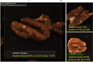
Al-enabled vision systems and software classify and identify acceptable nuts for placement on chocolates.
