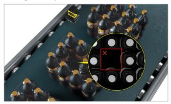
In-Sight 2D vision sensors detect the presence or absence of objects during final assembly.
