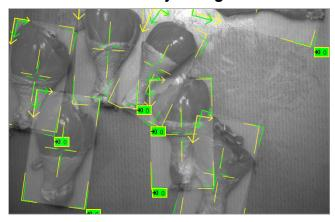
Al-powered vision systems identify meat cuts on conveyor, classify good or bad items, and locate coordinates for robotic picking.
