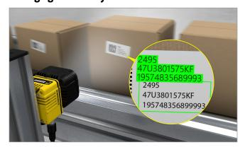
In-Sight vision systems and OCR vision tools read alphanumeric date/lot codes to ensure supply chain traceability.
