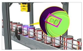
3D laser imaging technology quickly inspects aluminum cans on high-speed lines for defects.
