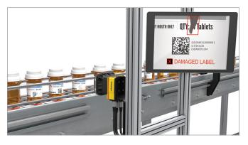
In-Sight vision systems with feature extraction technology use lighting and software algorithms to create high-contrast images which enhance the 3D features on a part. It catches errors and defects such as torn, ripped, or warped labels.
