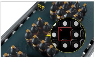
Cognex AI tools find complex features and objects by learning from annotated images. Self-learning algorithms locate different types of vessels or vials on very noisy backgrounds or other complex objects in bulk. To train the tool, the user provides images where the targeted features are marked.
