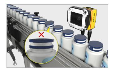
3D laser displacement systems optimize product quality by providing accurate, micron-level 3D inspection. A laser displacement sensor placed above open boxes uses 3D measurements to ensure that the cap on every bottle inside is properly positioned. Mis-assembled caps are flagged before the box is closed and placed on a truck for delivery. This helps avoid spills and quarantines defective product before it leaves the facility.
