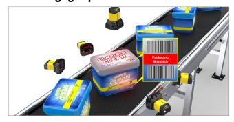
Image-based barcode readers can check that lids and containers match and accurately reflect package contents.
