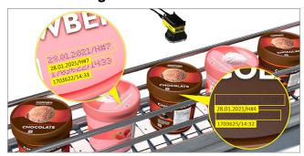
Reliably read text on packaging that changes in size, color, and orientation with Al-based OCR tools.
