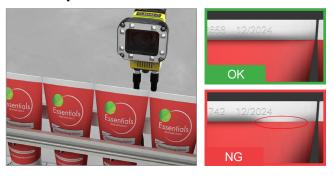
Al-based image analysis detects unpredictable defects.
