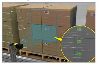
Barcode readers with expanded field of view technology scan pallet labels on arrival.
