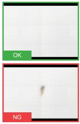
Machine vision systems inspect materials, such as diaper padding, for defects and inconsistencies in size, shape, color, and texture.
