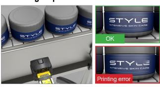
Vision systems identify torn, damaged, and missing labels with defect detection technology.
