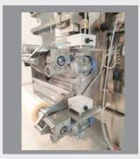
Quick release, drop-on, side loading, twin or tandem film reel air mandrel
