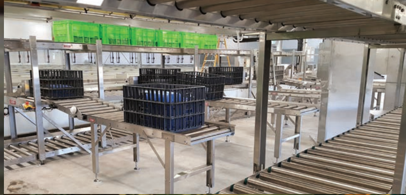
▼ Stainless steel, gravity roller conveyors
