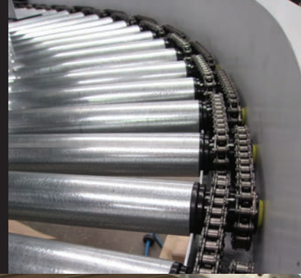
▼ Stainless steel, gravity roller conveyors
