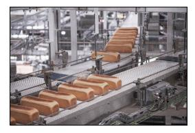
Fitted with Intralox Acetal and Polypropylene belts, we can provide these conveyors fitted with belts that have cleats or friction surfaces for angled applications.
