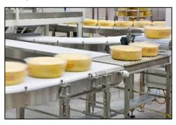
FlexLink WLX and X Series conveyors are the ideal solution for demanding production environments where contamination or chemical exposure present a potential risk. FlexCAM's stainless steel conveyor systems are specifically designed to meet the strict requirements of the food processing, pharmaceutical and personal care industries where hygiene and regular wash downs are critical.
