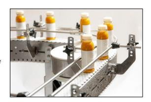
A full range of guide rails, supports, hoods and chain types are available along with disc bends for tight radius turns. We can also provide change part corner rails for different product sizes.
