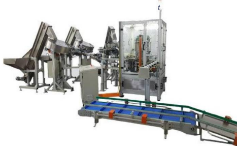
Fully Automatic Baggers with a Servo Drive Put Down Unit Direct from Airveyor
