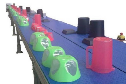
Mattop Belt Conveyoring
