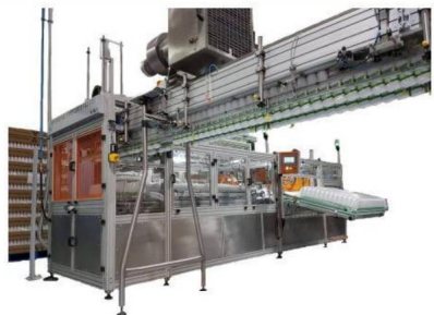
Fully Automatic Baggers with a Servo Drive Put Down Unit Direct from Airveyor
