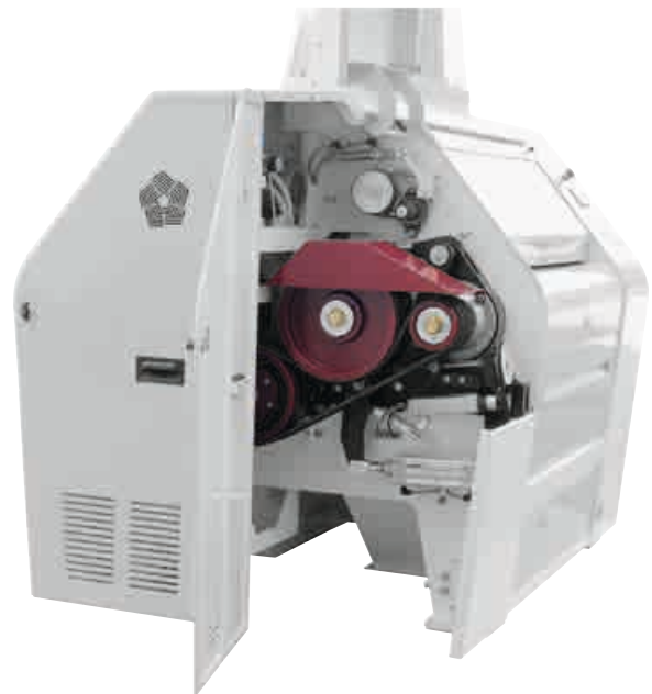
Integrated drive for format changes as a replacement for a handwheel
