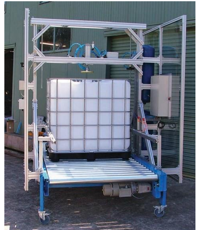
IBC Manual, Auto , with or without cage (constrained), camera for valve inspection
