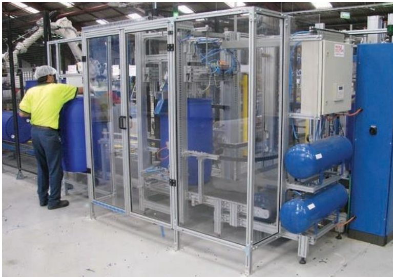
250LD manual or fully auto, Weighing, ORientation, Punching (WORP)+ testing
