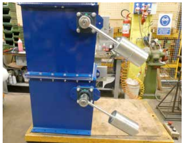
COUNTERWEIGHT VALVE: in this case, the activation of the flaps depends on the weight of the material.
