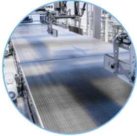
Small pitch belts for optimised transfers
