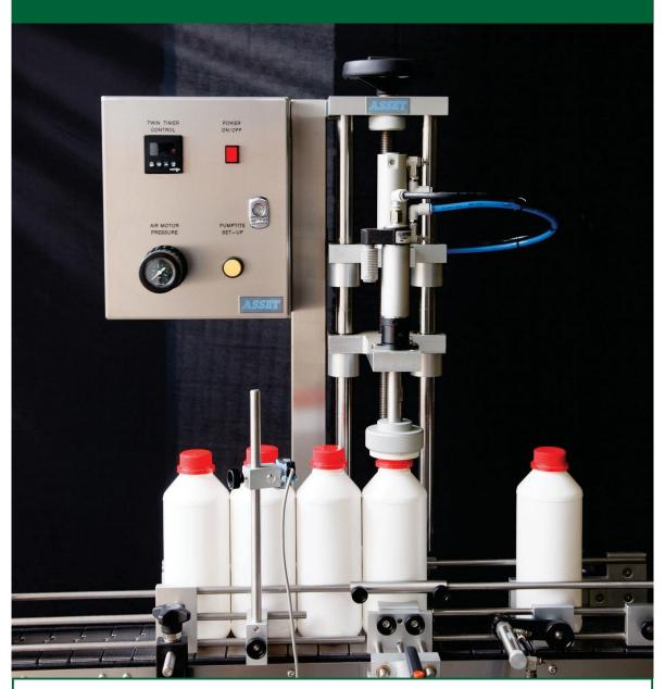
For the cap tightening of containers and bottles ranging in size from 10mm to 100mm
