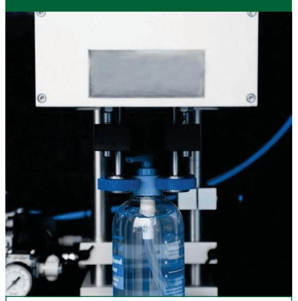
For the tightening of containers and bottles requiring trigger or pump dispensing caps
