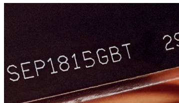
Laser mark on coated cardboard box
