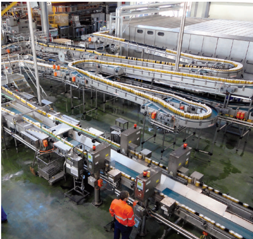
High-speed beer can conveying with control, mass flow merge and divider units
