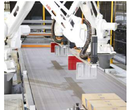
High-speed, high level with track and grip head (dynamic pattern forming)
