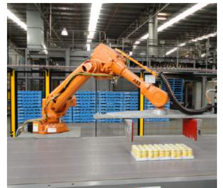
High-speed, low-level with track and grip head (dynamic pattern forming)
