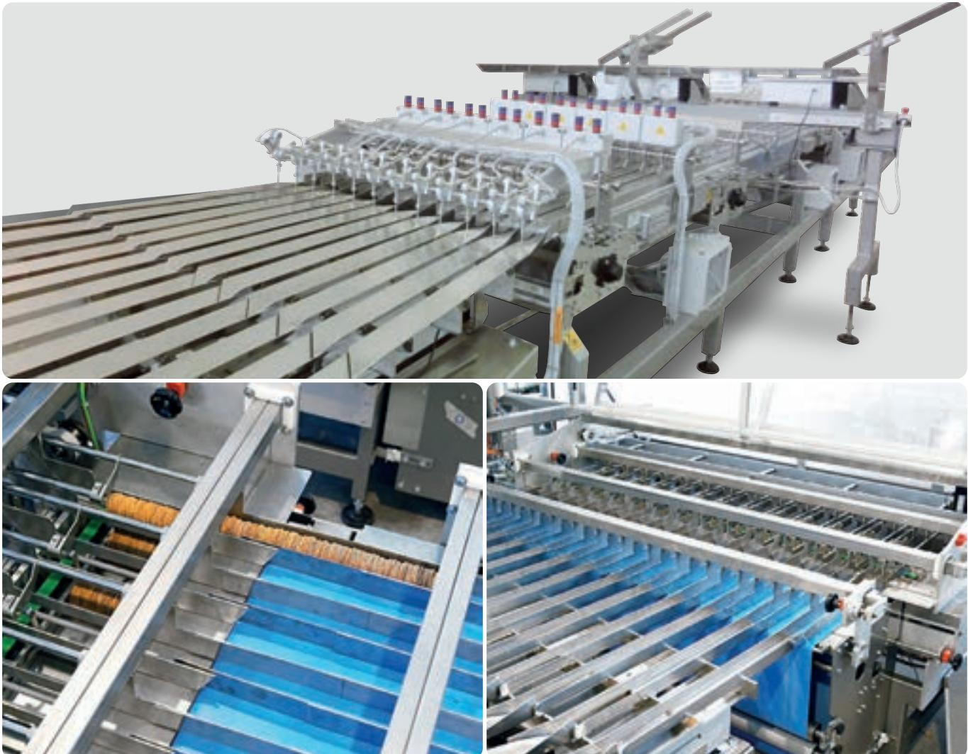
Automatic feeding system to take products from the processing line end, to buffer them, to control their quality, to prepare the volumetric portion and to feed the slugs on to the wrapper infeed.
