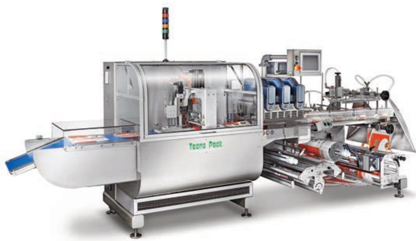
Electronic machine with bottom-mounted reel can be used for packaging fragile, irregular or heavy products, which need to be "carried" by the wrapping material.
