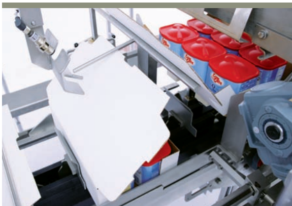
Servo-driven lowering principle
