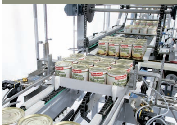
Tray transport chain and glueing station
