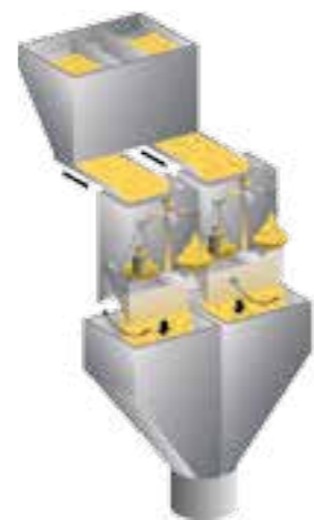
2 PV2 automatic weighing system
