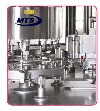
Self-adhesive rotary labelling machines for cylindrical, square, oval containers, etc. Possible types of labelling: Label, back-label, neck collar, shoulder collar, band, seals, etc.
