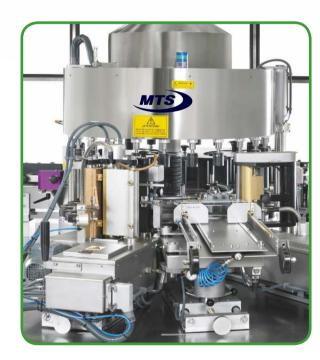
Hot-melt rotary labelling machines for cut and stuck paper or plastic wraparound labels for cylindrical, square, oval containers, etc.
