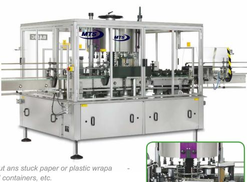
Hot-melt rotary labelling machines for cut ans stuck paper or plastic wrapa round labels for cylindrical, square, oval containers, etc.
