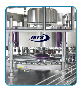
Cold adhesive rotary labelling machines for cylindrical, square, oval containers, etc. Possible types of labelling: Label, back-label, neck collar, shoulder collar, band, etc. Machines with guillotine type protection.
