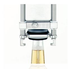
Level probe technology enables enhanced accuracy and flexibility to handle different bottle sizes without any changeover
