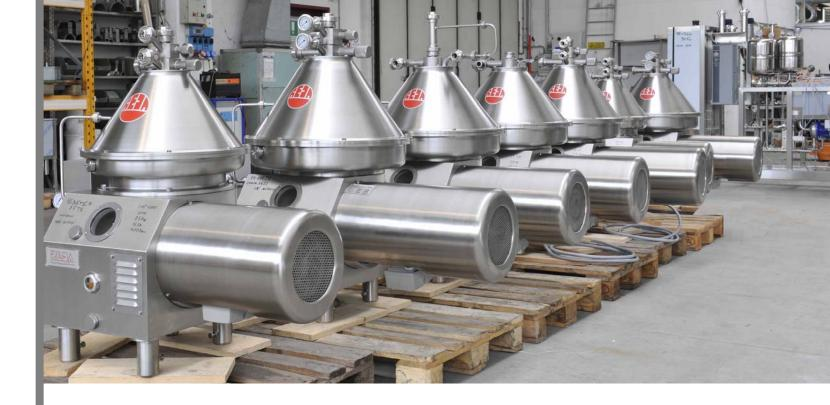
The PRS<sup>TM</sup> guarantees a full control of the separation process without any product damages: in fact, the centrifuge will perform highly effective ejections with an extended discharge time.
