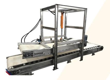
A Bag Flattener is an equipment which assists in the automatic flattening of the Bags/Sacks for ease of coding and palletization. The filled Bag/Sack with uneven shape is passed in between the two conveyors at the desired height and the Bag/Sack carries a uniform flat shape at the discharge end through compaction.
