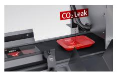
Identify leaks smaller than 0.3 mm using patented Quantum Cascade Laser (QCL)technology
