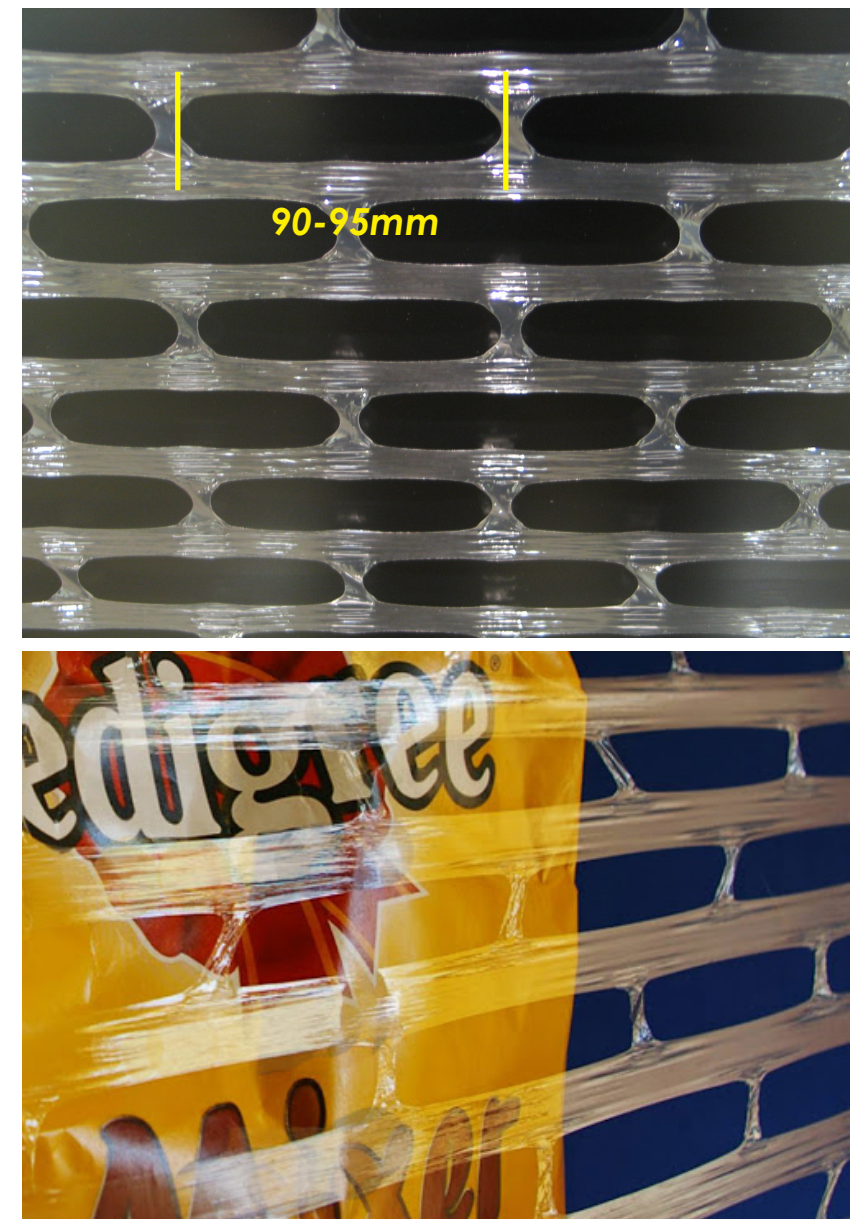
after film is stretched by PSE5100 wrapping machine
