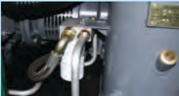
Lubricant filter assembly features a spin-on, full-flow, 12µ, high-efficiency components
