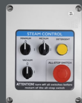
External control panel to command the belt cleaner functions
