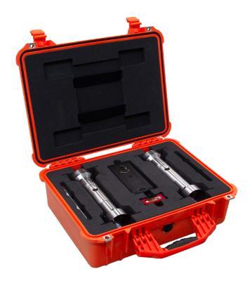
Digital core orientation system that provides directional characteristics of a geological core sample
