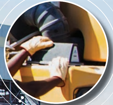
Proximity Generators mounted on machinery create electromagnetic field(s) around entire vehicle.
