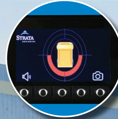
Driver is alerted when person or vehicle is detected within marker zones generated by Proximity Generator.
