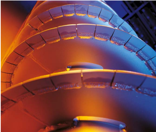
Tungsten carbide tiles mounted on the scroll conveyor prevent abrasion problems.
