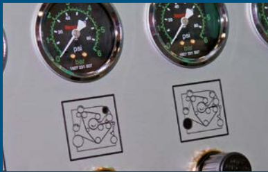
8. Air pressure operated paper tension setting
