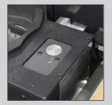
The tool length sensor is used to automatically measure the length of a tool and create an accurate tool length offset. This saves you time and ensures precise and consistent cutting depths with all tools.
