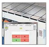
Auto zone management allows the router to operate in Live Deck mode which will automatically activate and deactivate zones according to the live position of the cutting head.
