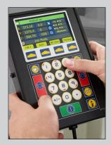
The AXYZ SmartConsole brings unprecedented ease of use, context sensitive menus, real-time display of machine status and many more time-saving, functional and productivity features. It provides a graphical preview and current status of a running job and allows program feeds and speeds to be changed without pausing the program
