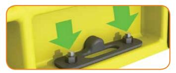
3. Check linking plate bolts are tight on top.
