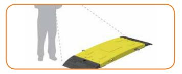
1. Check top surface of Road Plate for signs of damage.
