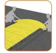
**10.** Repeat previous step until **11.** Use M16 bolts to secure entire trench is covered by inner Road Plate sections.
