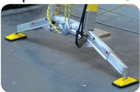
Step 4 Attach rope tethers around pole or to structure. Apply tension.
