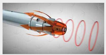
The crowned head is perfect for incohesive, rocky and densely packed soils. The tip of the cutter bit starts a preliminary pilot bore and the crown cuts the soil. The crushed soil is relocated to the ducts, lead to the rear and displaced outwards. Due to this working principle the crowned head features highest precision and penetrating power, even if the ground is hard and stony. The pressure cone generated in front of the crowned head is bundled and targeted.
