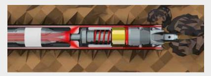
During the second stroke, the bore head moves freely in the bore hole and the piston aims the impact right up to the casing. The impact power of the piston is concentrated on the casing and the complete machine (with the pipe attached) moves up from behind.
