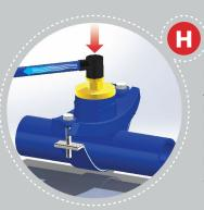
FIT THE NEW FERRULE SERVICE AND REMOVE THE SHUT OFF BLADE (22) CLEAN AND DRY EQUIPMENT PARTS AND PLACE INTO THE CUSTOMISED HEAVY DUTY TRANSIT BOX (23) FOR SAFE AND SECURE STORAGE.
