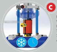
FIT THE FREEZER JACKET (11) WITH VENT TUBE AND FREEZE USING CO2 GAS SUPPLY FITTED TO THE DRIVE SHAFT FOR 2 – 4 MINUTES. FREEZE LASTS APPROX. 15 MINUTES.
