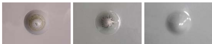
PAINT: (FAILED AT 4.5 Newton Meters)
