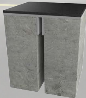
If expected movement is greater than 2mm, then decouple with plastic strip that is 4x the original joint size
