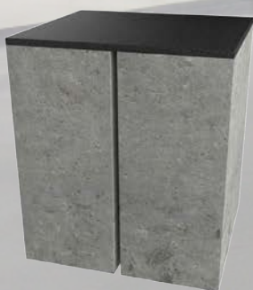
Cracks with movement under 2mm are sprayed over directly
